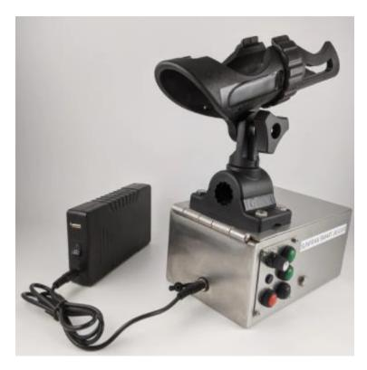
Here is how it works. There is a rod holder mounted on top of a small metal box. An electric motor pivots the lid of the box up and down. A small knob on the side of the box allows you to motor the lid up and down, and then record and save the motion using 'A' and 'B' record buttons.
